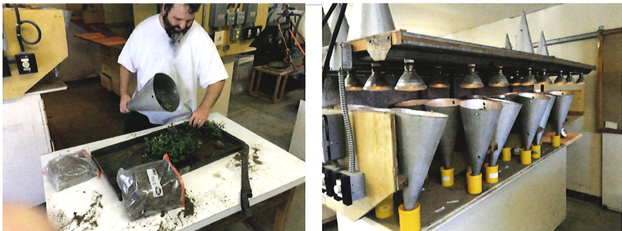
Figure 7. Slitting 1 gallon sample to fit in Berlese (left) and final set up of Berlese funnel bank.
